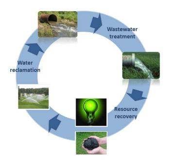
The anaerobic biological process applied in this technology transforms the organic matter into biogas – a renewable source of energy – with low sludge production. Membrane filtration disinfects low-loaded wastewaters at ambient temperature.
